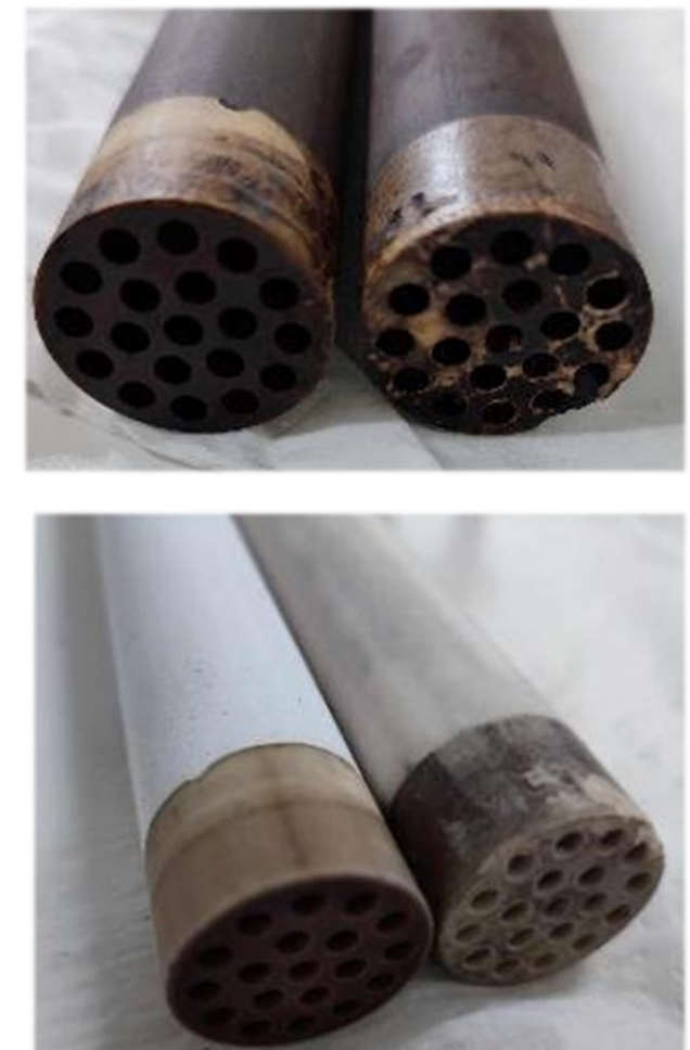
Atech membranes before and after cleaning with NaOH
